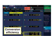
Measure the power conversion efficiency of primary and secondary systems
